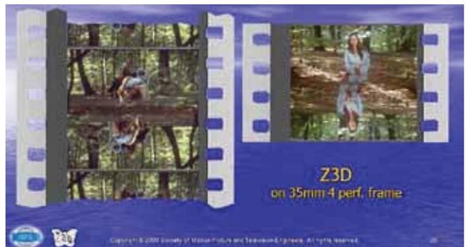
**Figure 9.** On standard 4 perf frame, each image occupies 2 perforations in height. Frames from *Dracula Returns* Z3D demo. (Directed and photographed by Z.P.)
